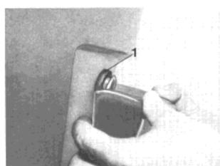
Installation instructions: Seal off attachment bolts between the body and underlay plates with sealing compound.
