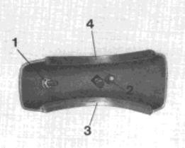
Unscrew nuts (1 and 2) and remove rubber pad. Installation instructions: Ensure correct seating of underlay (3 and 4).
