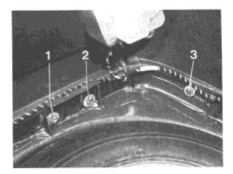
Installation instructions: Do not forget rubber spacer piece (1) between bumper and body.
