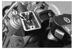
Refill oil, until it is discharged from the bore of the master cylinder in a bubble-free state. Make sure that the oil does not overflow.
