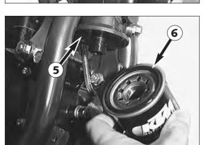
Clean sealing surfaces on the front pipe 6, fill new fine screen filter with engine oil, and oil rubber gasket 6. Replace fine screen filter and screw it back in place, your bare hand will do.
