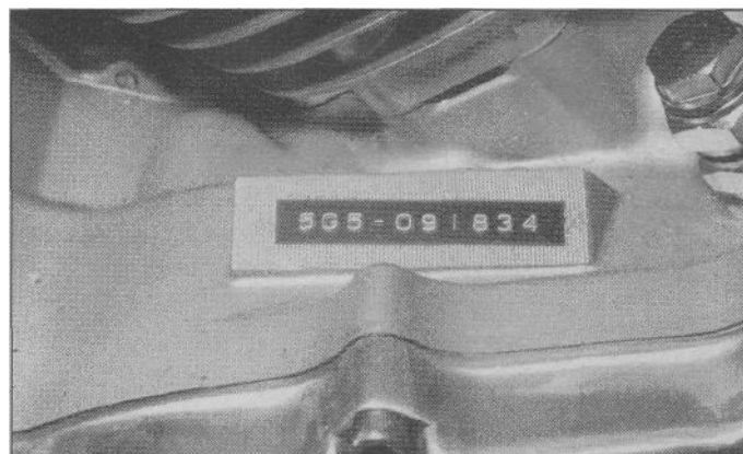
The engine number is stamped in the right side of the crankcase
